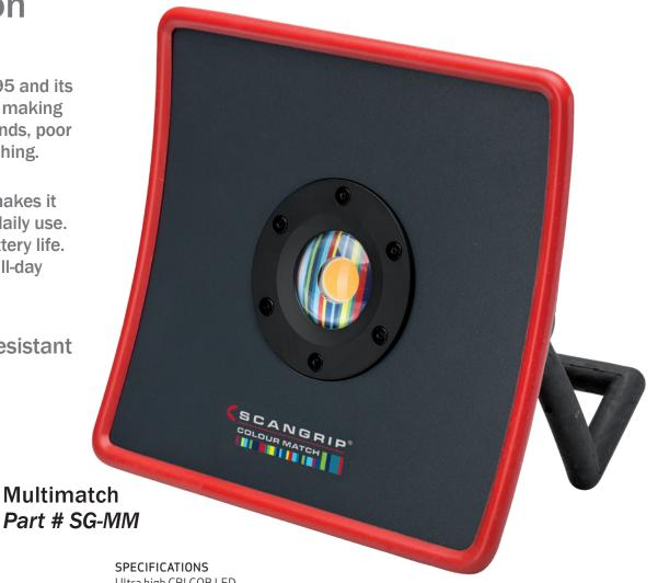
Ultra high CRI COB LED 95 CRI 4500 KELVIN 3500/1400 lux (step 1/step 2) 2000/600 lumen (step 1/step 2) IK07 IP67
