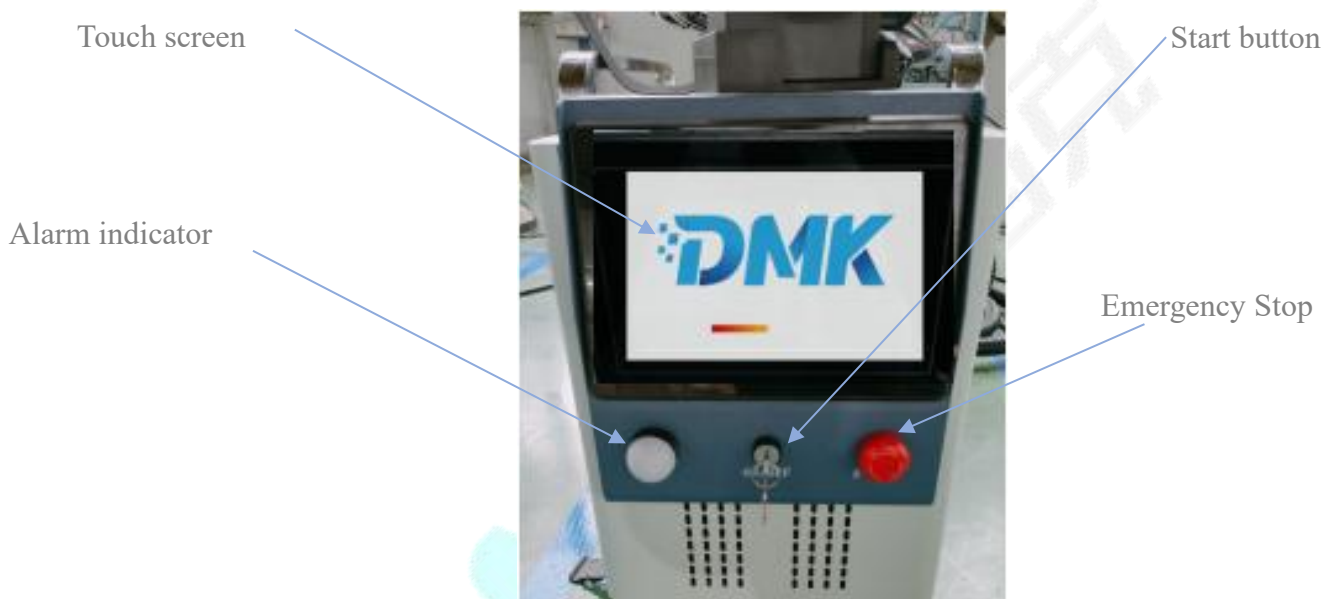
Fig3.3 Front operation panel of DPL-300W
