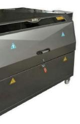
**Stainless Steel** 150x110x140 cm (Machine Dimension) **Basket Diameter 90 cm** Loading Height Max. 45 cm Loading Weight Max. 300 kg Tank Capacity 80 lt. **Mechanic Door Automatic Cleaning Rotating Basket Reducer High Pressure Cleaning 2.5 bar High Pressure Cleaning Nozzles** Water Temperature Control Water Heater 90 Deg. **Discharge Station Cleaning Timer Control Oil Skimmer**
